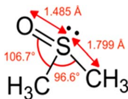
Figure 12. Chemical structure of DMSO. [Color figure can be viewed in the online issue, which is available at wileyonlinelibrary.com .]
